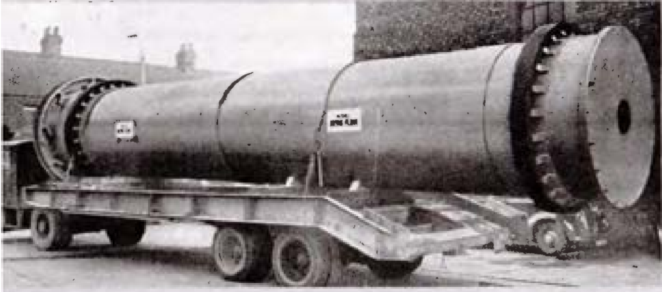
◀ Rotary Calciner 6' dia. × 40' long, weighing 24 tons, in transit
