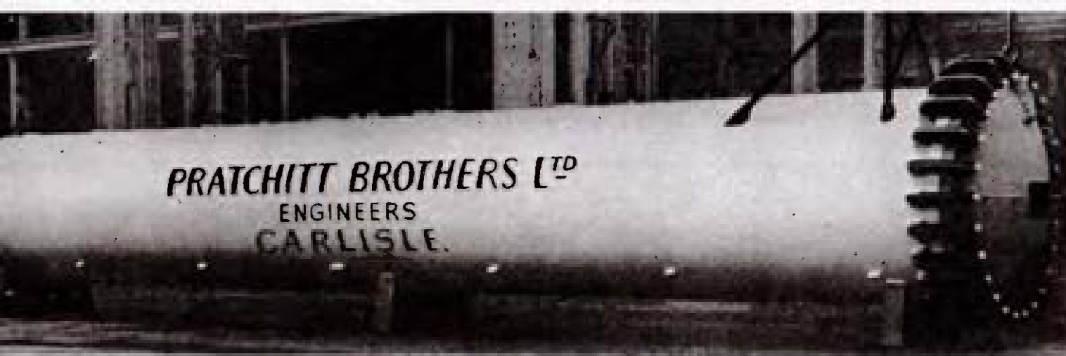
▲ Timber Pressure Impregnating Cylinder 6' dia. × 40' long
