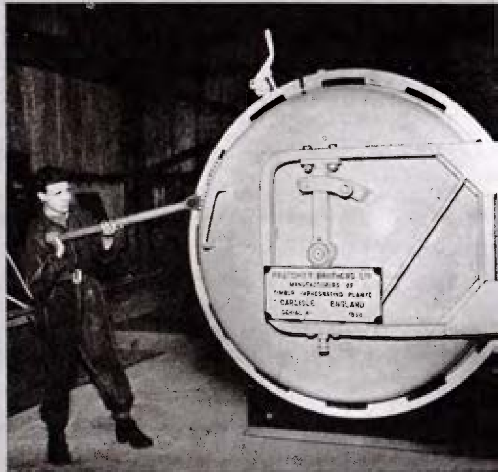
▲ Quick Opening Door Mechanism being used on Timber Pressure Preserving Cylinder
