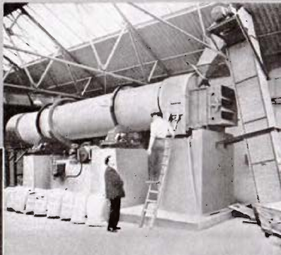
Rotary Dryer installed in a Chemical Works, for handling Saltpetre.
